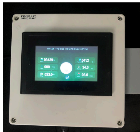
Figure 3: Active Display Screen showing real-time sensor readings.
