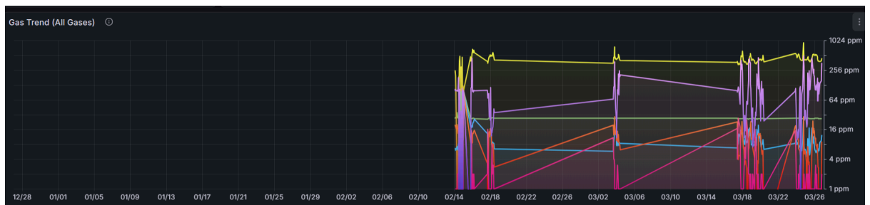
Figure 10: The Gas Trend (All Gases) graph showing historical ppm levels.
